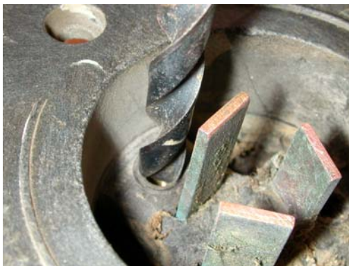
Drilling out the rivets
