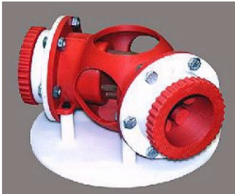
Fig. 4.2. Fused deposition modeling (FDM) concept model of a pin drive mechanism. (Courtesy, The Innovative Manufacturing Centre, UK.)
