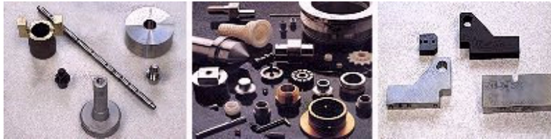
Fig. 3.1. Simple geometric shapes are best fabricated using subtractive CNC.
