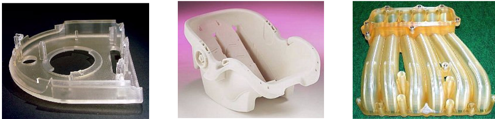
Fig. 3.2. Complex or compound shapes are best fabricated using rapid prototyping. (Courtesy, L-R: Cadem A.S; Z Corp.; Cadem A.S.)
