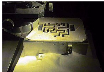
Fig. 3.4. Injection mold with conformal cooling fabricated by Laser Engineered Net Shaping™ (LENS®) (Courtesy, Optomec.)
