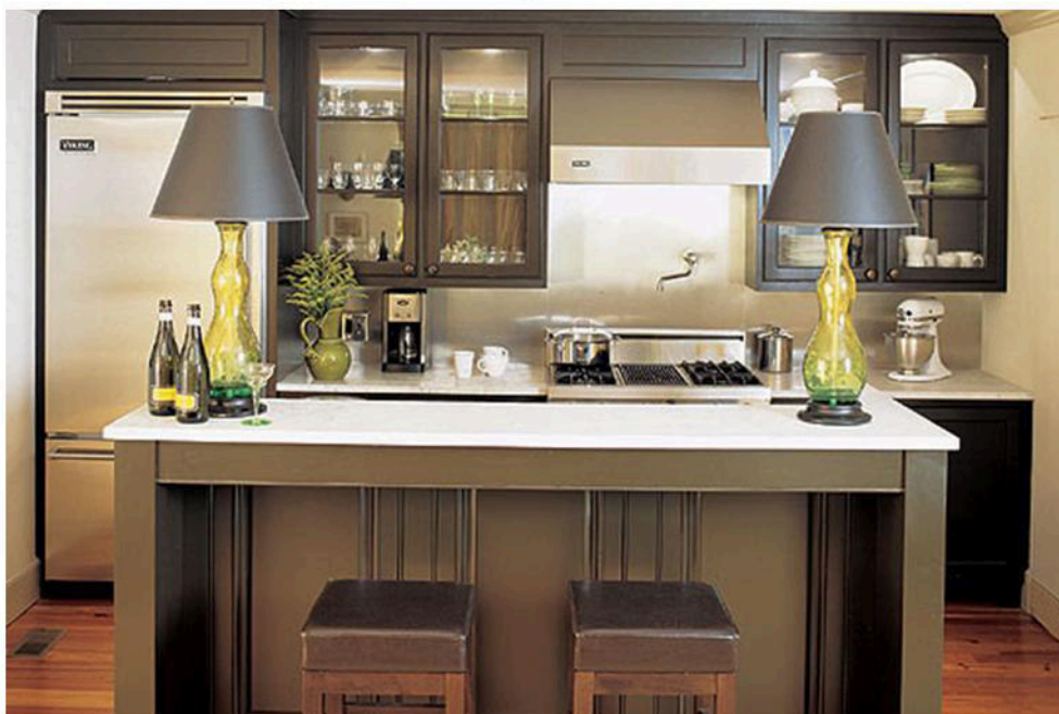
A 42" high breakfast counter conceals sink on the 36" high side of island. Carrera marble top and stainless steel back splash. Homemag.com
